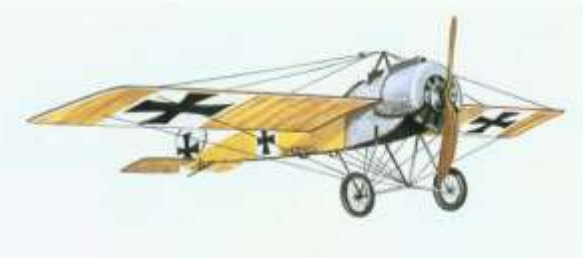
Oswald Boelcke and his Fokker E.III, built 1915, powered by Oberursel UI 9-cylinder air-cooled rotary 100 HP engine, weighed 1,342 lbs., maximum speed of 88 MPH, maximum ceiling of 11,500 feet, 1 synchronized Spandau machine gun
